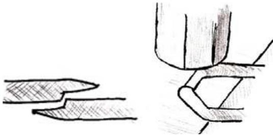
Figure 11: Final position before welding
