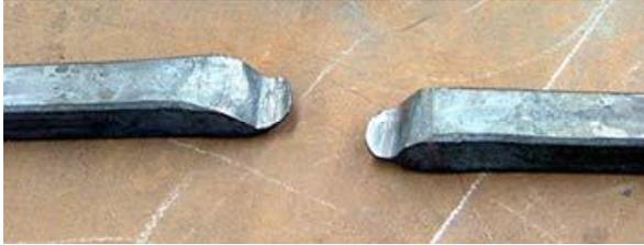
Figure 5: Two scarfed bars ready for welding
