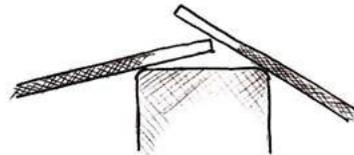
Figure 3: Positioning bars for welding
