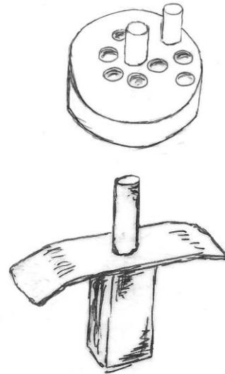
Braze or weld the square stock to the middle of the 1" flat stock. Mark & drill a 3/8" hole so when it passes through the flat stock it will be centered in the 1" square stock. Drill 3/4" deep. Place the vise pin holder in your vise and hammer the flat tabs to conform to the jaws. In a vise the pair of pin holders can be easily moved and secured in the position you need.
